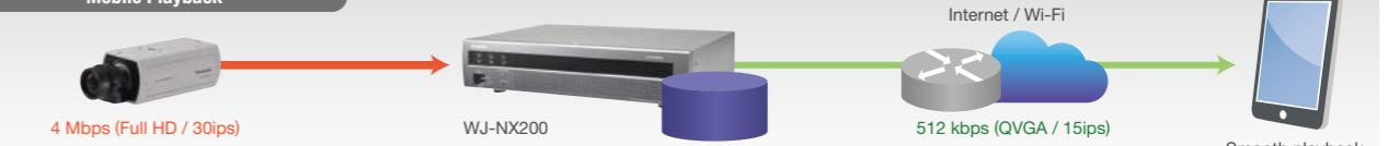
WJ-NX400 / WJ-NX200 / WJ-NV300 can transcode image size/bit rate to fit the customers environment, and stream it. This mode can be used by WJ-NX400 / WJ-NX200 / WJ-NV300 only.
