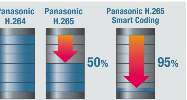
"Smart Coding" provides over 95% reduction in total file size when compared to "H.264"
