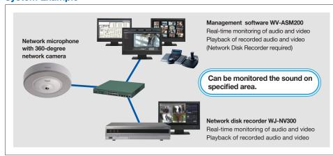
Pick up clear sound of specified area in noisy or acoustically live environments.
